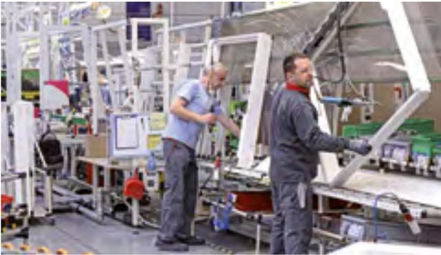
**Production of wood-polyurethane windows in the window factory in Namysłów.**
